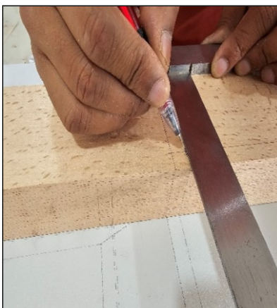
Using try square for front face marking
