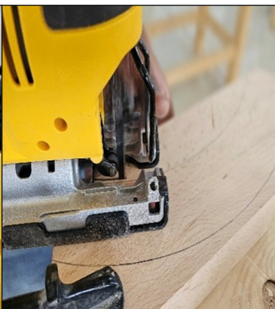
Cut the arc using jigsaw
