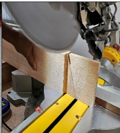
Proceed with angle cut using miter saw
