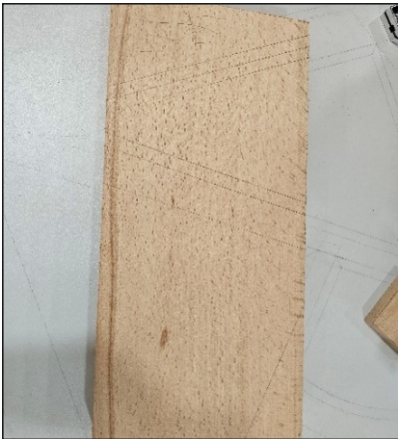
Place the material on drawing board and mark all lines on the material
