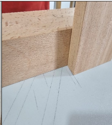
Using a right-angle block for transfer measurement
