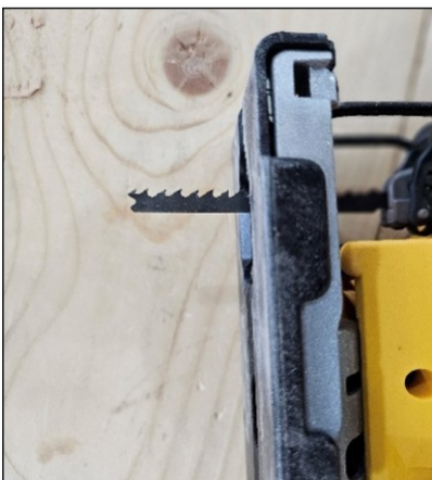
using jigsaw and a rough blade for arc material cutting
