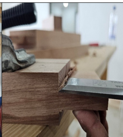
Now using chisel and clean the side parts
