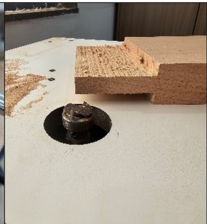
Then use table router and set dado bit to clean the tenon surface
