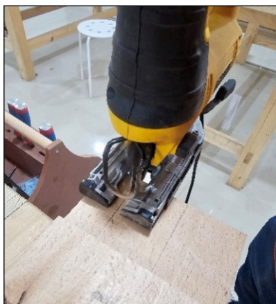
Using jigsaw or band saw, for cutting tenon side parts
