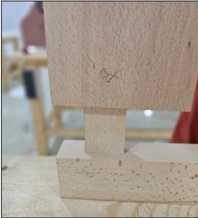
joint fitting check
