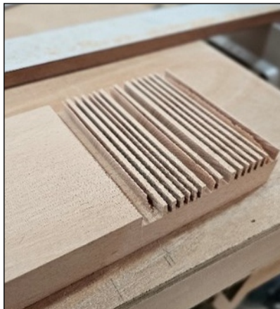
Final miter saw cut
